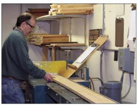
**Making blanks** — Craftsman Waldemar Giro cuts blanks for an upcoming job. After the blanks are cut, a label is affixed to each blank identifying the piece and the job. From here, the blanks go to a clamp carrier.
